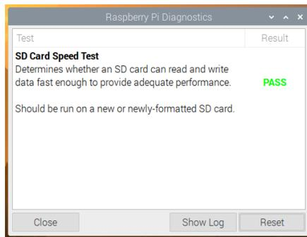
We are testing against the A1 specification, which requires a sequential write speed of 10MB/s, 500 random write operations per second, and 1500 random read operations per second; we run the test up to three times. (Tests of this nature are liable to errors due to other background operations access-
